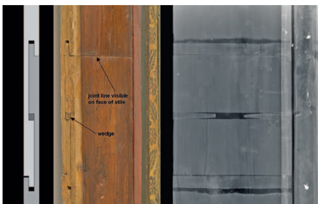
Fig. 4 Tenoned scarf joint of vertical stile: drawing of side view (left), photograph in three-quarter view (center) and X-radiograph taken from the front (right). Drawing: Beth Edelstein, photograph: Mechthild Baumeister; X-radiograph: Timothy Hayes, all © The Metropolitan Museum of Art.
