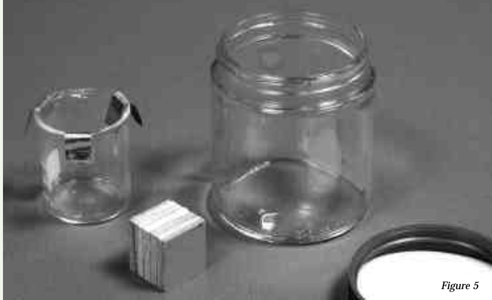
Figure 5. Elements of a three-in-one set-up for testing a sample of wood laminate.
